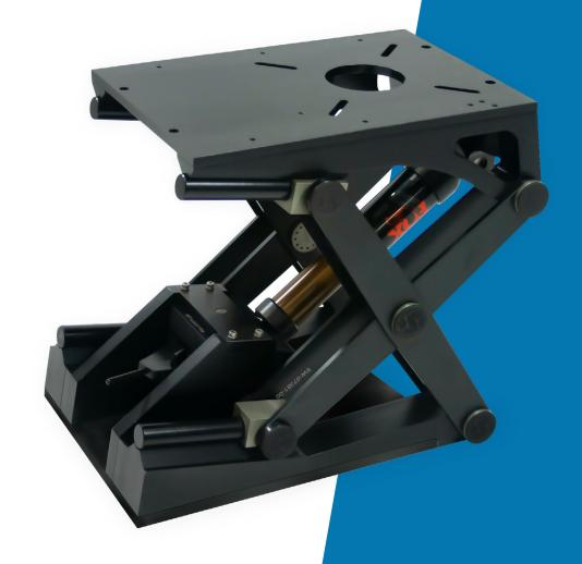
The S6 is a purpose-built suspension module with a fully integrated height adjust, actuated with a ratchet mechanism for precise adjustability. It provides 5.5" of travel to mitigate the shock of 6g impacts for occupants up to 300lbs. The height of the S6 Suspension Module is 10" in its lowest position and 13" in its highest.
